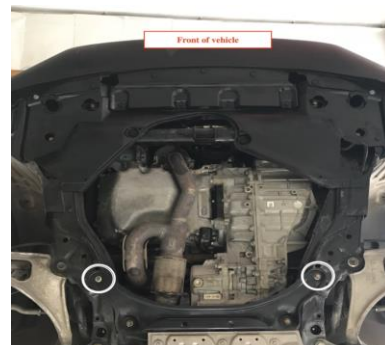
2. Locate and remove the two 14mm cross brace bolts. (Shown above)
