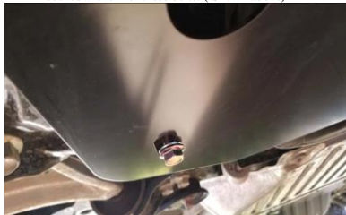
3. Lift the skid plate in place and insert the 14mm cross brace bolts (with washers) back into place loosely allowing movement for the skid plate.
