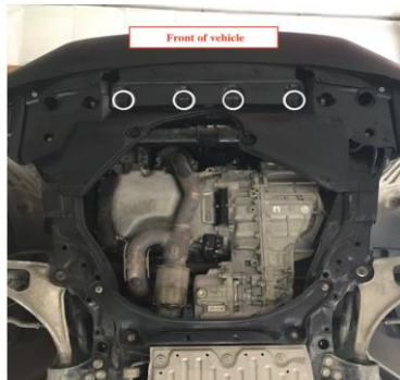
1. Start by locating and removing the OEM bolts. Use a 10mm socket/wrench for these bolts. ( Shown above)
