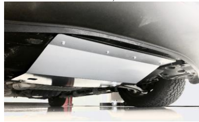
4. Using the provided 10mm hardware, locate the front holes and insert the provided hardware loosely allowing enough movement for adjustments.
